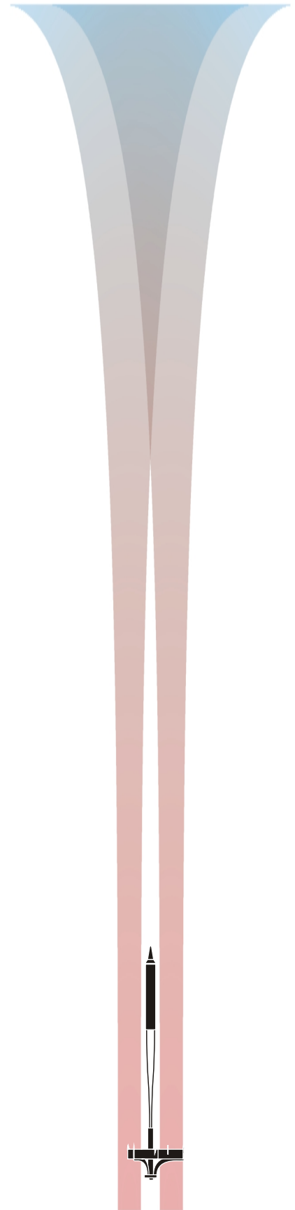
As speed increases the depth of the magnetic field increases as does its distance from the ship
